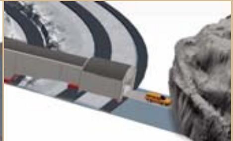
The movable test track allows us to test our vehicles on various outdoor surfaces. As the illustration shows, it even provides the opportunity of crashing into solid Swedish bedrock.
