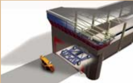
This fixed test tunnel is used for collision tests inside the center, and for rollover tests outdoors.
